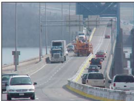
Figure 2. Moveable Concrete Barrier and Transport Machine
