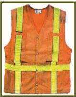
Characteristics: little or no reflectivity, and soiled and faded material.
