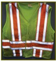
Characteristics: Good reflectivity but has some soiling and light fading of material. \*Note: This picture was taken with a flash and simulates nighttime conditions.
