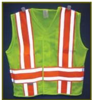
Apparel that is used but is in likenew condition is characterized as having excellent color contrast, excellent reflectivity, and is not faded or soiled.
